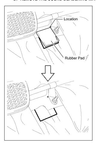
1. Temporarily place the rubber pad on the floor panel as shown, and outline the pad on the sound deadening material with a ball point pen.
