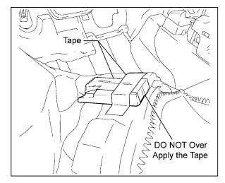
b) Secure the **NEW** upper tibia pad to the lower tibia pad, by applying the industrial tape to the locations shown.
