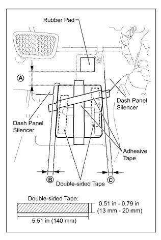
In the event the lower tibia pad has detached from the carpet, position the tibia pads on the floor panel and secure them using adhesive and double sided tape as shown.
