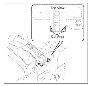
b) Using a reciprocating saw, cut the corners of the pedal.
